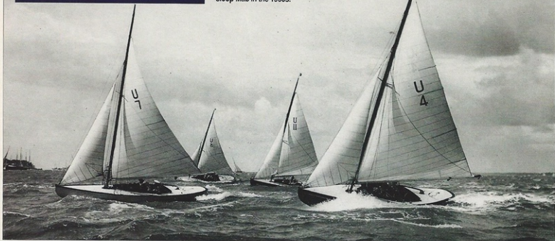
Main picture: A shoal of Seaview Mermaids reach for home during Cowes Week, 1930. U4 has one turn of the mainsail on the boom, and her crew are perched on the weather deck, while U7 has two rolls reefed and her crew are sitting comfortably in the cockpit: two opposing philosophies of racing. Inset: The 1913 Woodnutt sloop Mab in the 1960s.
